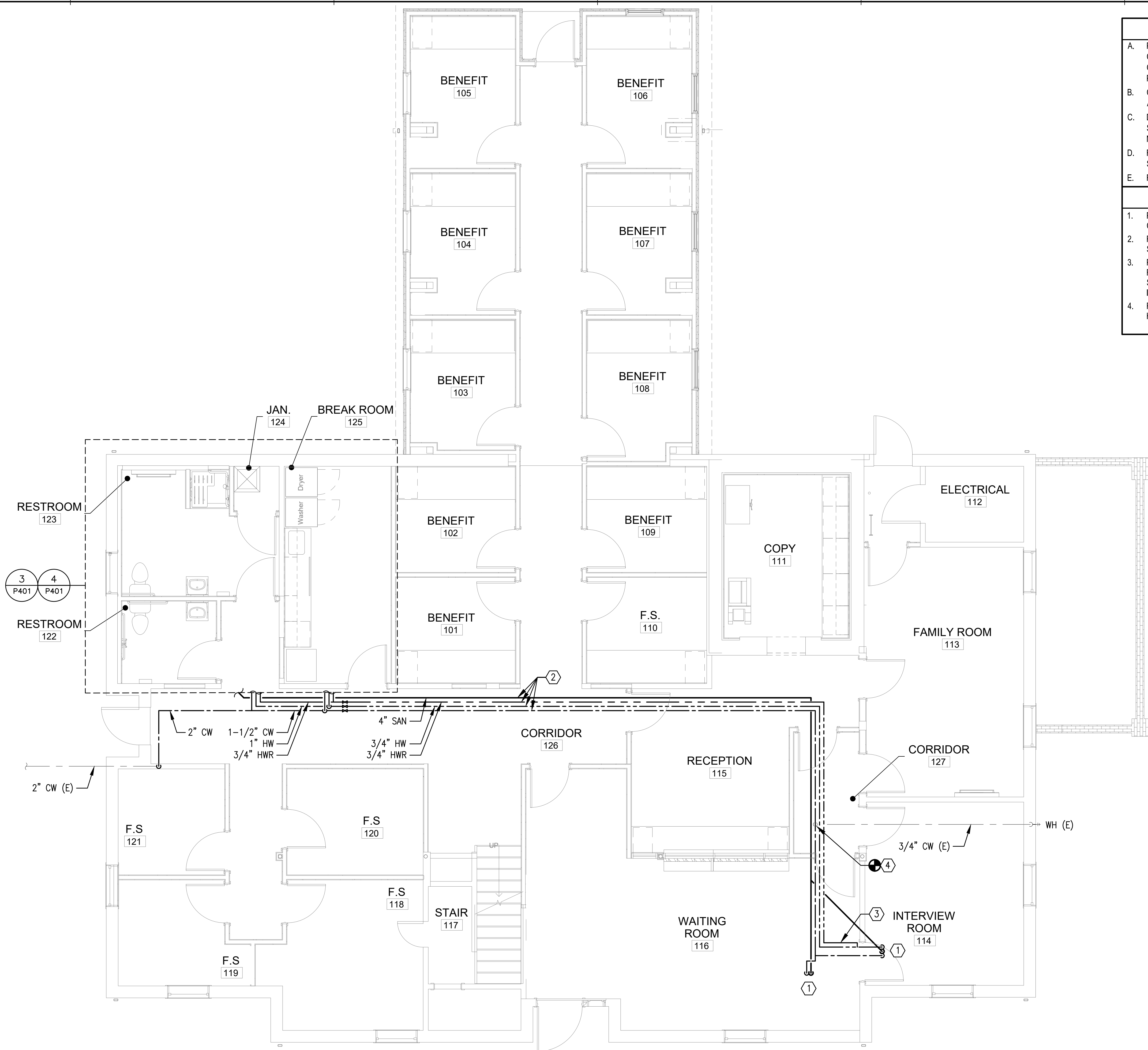
1 PLUMBING NEW WORK PLAN - FIRST FLOOR P101 1/4" = 1'-0"
